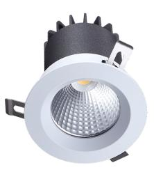
The Corona Mini LED downlight has a 70mm diameter bezel whilst using a CREE LED engine. The heatsink is constructed from die-cast aluminium complete with aluminium bezel and reflector.
