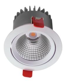
The Corona Adjustable LED is a 120mm diameter downlight which uses a CREE LED engine. The heatsink is constructed from die-cast aluminium complete with adjustable aluminium bezel and reflector.
